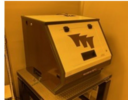
Laser Writing System 1 \mu m res – 385 nm wavelength
