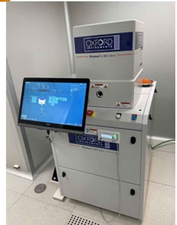
Plasma Lab 80+ Oxford ICP Etching; Deep Si Cryo and Bosch Etching
